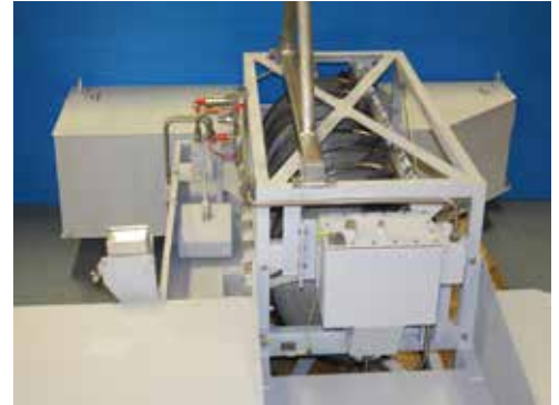
Above: Float valve controlling the transfer pump
